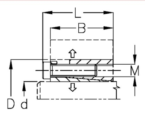
B mm = 33.0d H8 mm = 42D mm = 75Fit tolerance = Aksel h8, Nav H8 F kN torque = 105L mm = 41M mm = M8P N/mm2 surface pressure on shaft/hub = 190 Surface roughness = R? ?  $3.2 \mu m$ T N m torque = 2200Ts N m bolt tightening torque = 35
